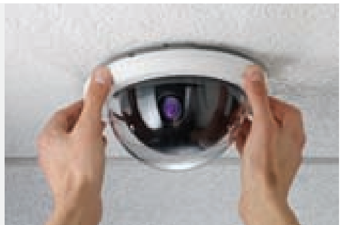
And replace the bubble.
