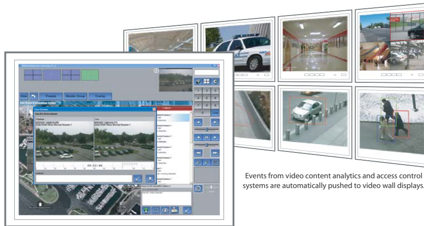
The NetSwitcher controller interface, shown with the events list and investigation panels
